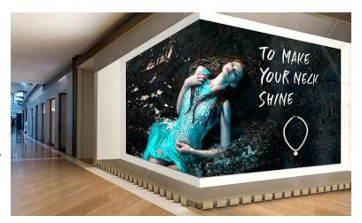
low-profile and lightweight design with an edge thickness of 37.5mm making it ideal for spaces where space is a concern. The display is capable of 800 nits of brightness and uses the widely used 16:9 aspect ratio, minimizing time and costs associated with content redevelopment. The cabinet also offers front servicing, making for easy maintenance. The Ultra Slim LSCB Series is EMC (electromagnetic compatibility) Class B certified, meaning it is not only perfect for
